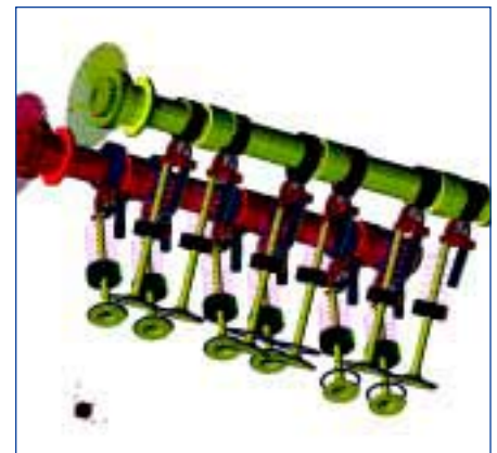
A 3D finger-follower valve train system with deformable rockers, camshafts, springs, and valves.
