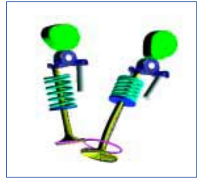
Valve train view of a single intake & exhaust pair - with deformation emphasized.
