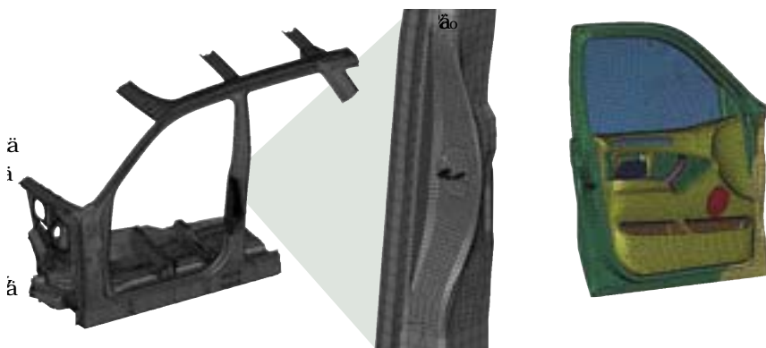
Cut-out and refined mesh in the critical area around the lock hook.
