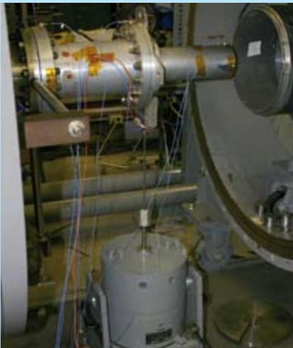
Vibration responses of the MSFC rocket nozzle test facility served as input for creating a structural dynamic model of the facility in LMS Virtual.Lab.
