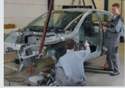
1 The car body model is modeled by measuring FRFs at all suspension-body attachment points.
