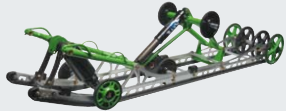
In redesigning a snowmobile suspension from a torsion spring to a coil spring configuration, Arctic Cat engineers studied stiffness and load-carrying capabilities using Virtual.Lab Motion to quickly perform multiple iterations of a suspension analysis that included different pivot locations, linkage lengths, motion ratios, and spring rates.
