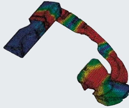
In predicting radiated noise with LMS SYSNOISE, engineers start by building acoustic models based on CAD geometry. The primary focus of their simulation is typically the air intake system, including the plenum, air box and inlet assembly shown here as the colored parts fastened to the top of the four-cycle snowmobile engine.
