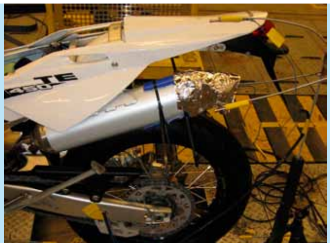
More than 20 microphones were located around the individual motorbike elements to record the noise levels.
