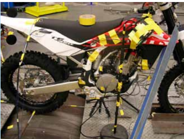
The bikes were installed in LMS’ semi-anechoic chamber equipped with a dynamometer to reproduce road conditions.
