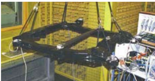
To validate the FBS simulation approach, Opel engineers characterized the body and subframe individually through FRF measurements, and compared the predicted vibroacoustic responses of the experimental FBS model with responses measured directly on the assembly.
