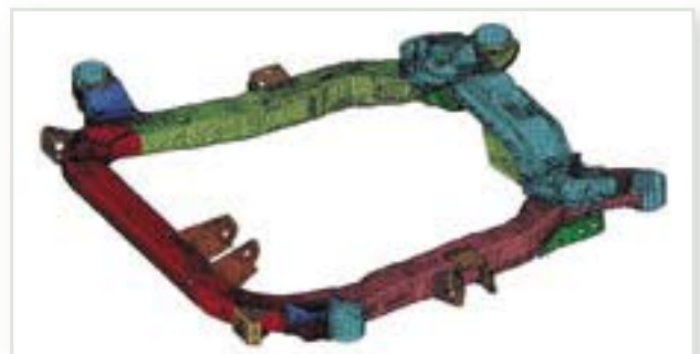
In a second step, they replaced the measured subframe FRFs with simulated FRFs obtained through FE modeling. Its ability to combine experimental and simulated FRF component models allows FBS to perform vibro-acoustic simulations early in the development.
