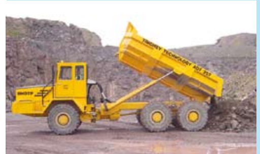
Six-wheel drive and good maneuverability enable articulated dump trucks (ADTs) to haul heavy loads over extremely uneven terrain.
