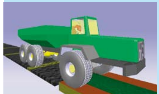
LMS Virtual.Lab allowed the simulation model to be “driven” over virtual terrain surfaces at various speeds to determine driver vibration levels defined by ISO 2631.
